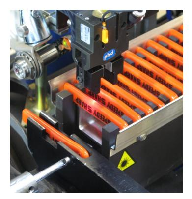
Hole is drilled in the Speedy Sharp handle before the tool is inserted.
