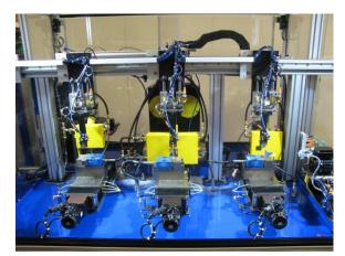
Three grind stations are used to finish all sides of the Speedy Sharp.
