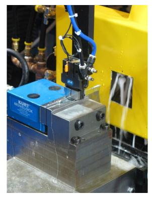
After grinding the sides of the carbide, part gripper moves tool to the next grinding station.
