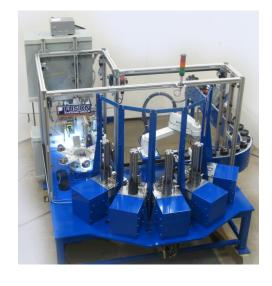
Scara Robot places piston into third ring insertion station.
