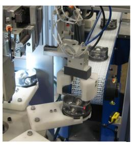
Pick and place unit removes the completed piston from rotary table fixture and transfers it to the discharge conveyor
