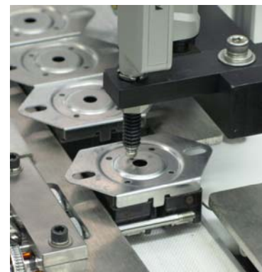
Contact probe verifies height of case subassembly.
