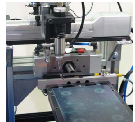
Dispenser applies sealant adhesive to display tabs.
