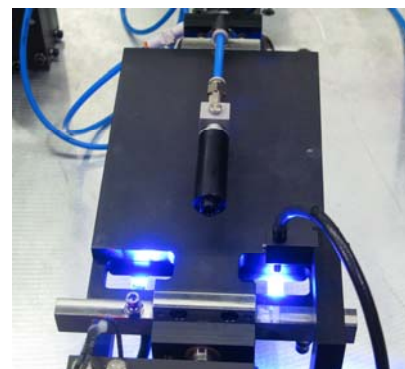
UV light-curing spot lamps affect tabs without disturbing active display area.
