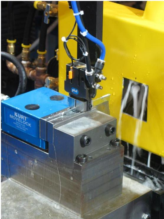
After grinding the sides of the carbide, part gripper moves tool to the next grinding station.
