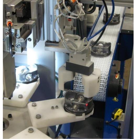
*Pick and place unit removes the completed piston from rotary table fixture and transfers it to the discharge conveyor*
