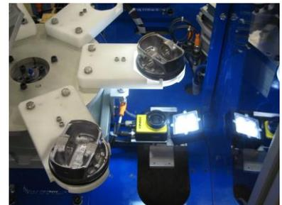
The system has two vision camera stations. The first camera station utilizes a Cognex In-Sight 7200 Camera with PatMax, which includes a 16mm adjustable focus lens with a white LED light. The first station looks for the identification marks on the piston and top and second compression rings to ensure the correct piston is loaded/assembled and the compression rings are oriented/positioned correctly.
