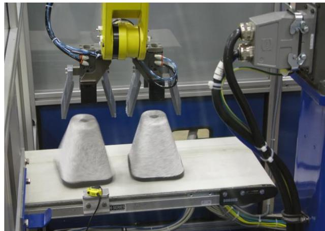
*Robot places completed shell assemblies onto discharge conveyor.*
