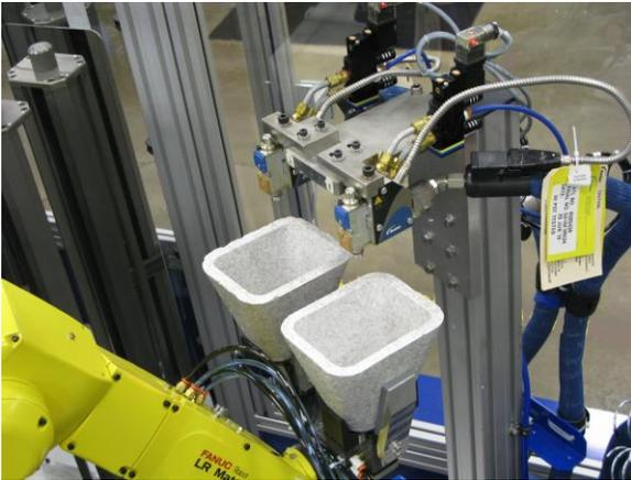
*Nordson Hot Melt Glue Applicator dispenses beads of glue to cover shell surfaces.*
